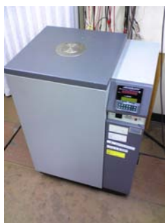
電気炉 :Hart 9115 Control panel: Bob S619p
