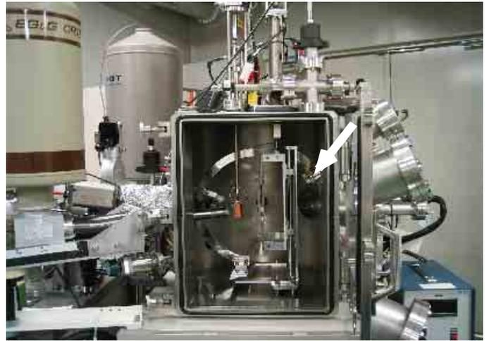
Photo.2 Inside of ion beam analytical chamber. A white arrow indicates a detector for ERDA and PESA.
