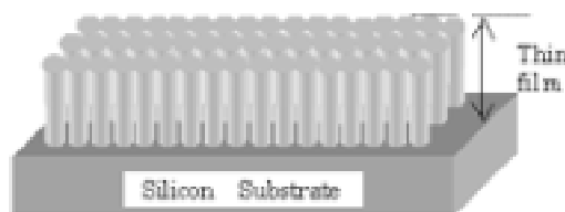
Fig.4 Cross sectional micro-structure model of deposited Al thin film.
